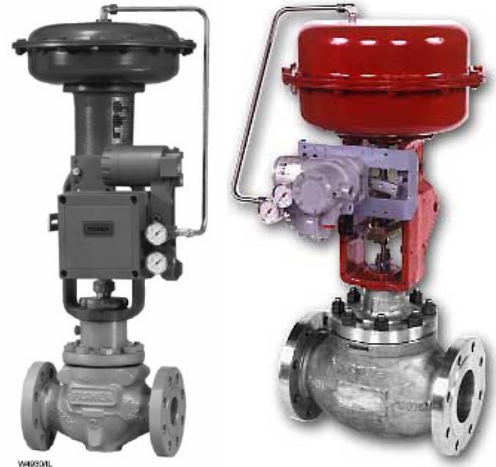
Globe Valve with Spring & Diaphragm Actuator & Electro-Pneumatic Positioner
