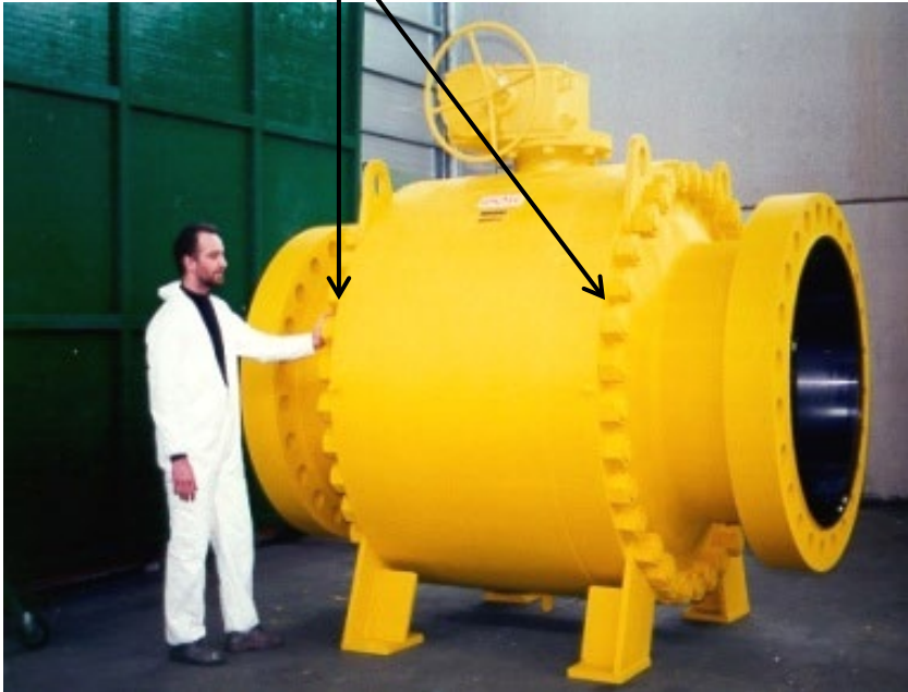
Side entry bolting
