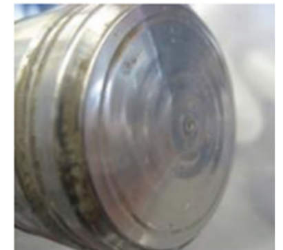
Pressure sensor diaphragm deformed due to H 2 ingress
