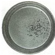
Hydrocarbon Dew Point
